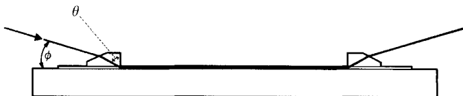
Fig. 3. A schematic showing the prism couplers into and out of the thin film, shown enlarged on the surface. The external angle \phi is changed by rotating the substrate on a rotating table. The related internal angle \theta changes the propagation constants k_z to match each mode.
